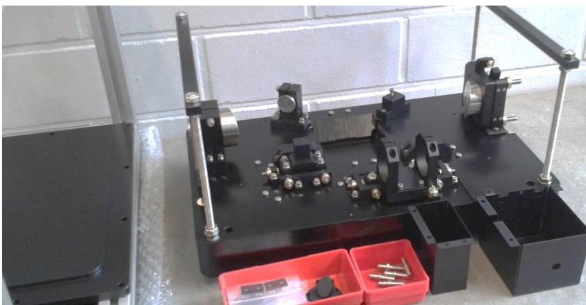
Mechanical parts installed on the breadboard and the cover plate of the inner box.
