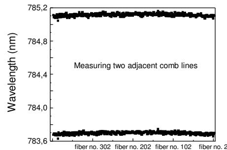
Astro-comb identifies calibration shifts due to irregularities in the fiber feeding of the spectrograph.
